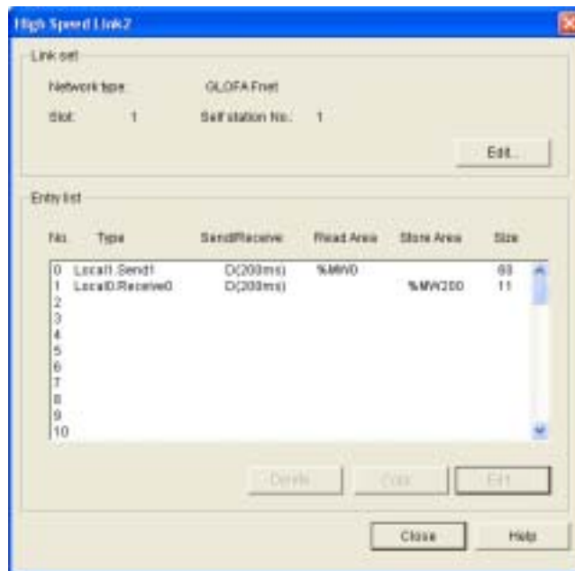
[Figure 12.1.27] High Speed Link network type, slot no. and station no. settings
