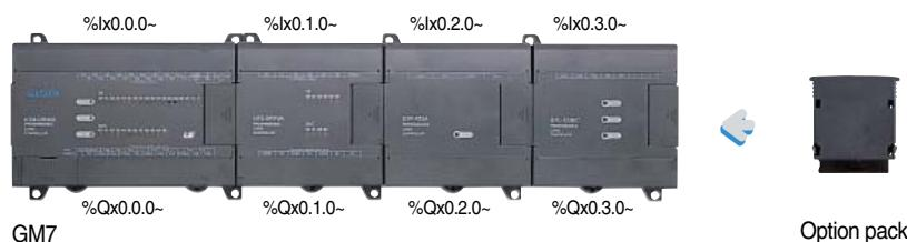
\* I/O assignment applies to digital expansion module. For example, if an analog module is used at the 1st expansion and digital I/O is used at the 2nd expansion, then, the input of 2nd expansion module is from %Ix0.2.0 and the output is from %Qx0.2.0 And I/O assignment of GM7 and GM7U is equal
