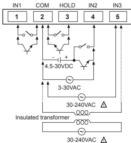
※ Please use reliable contacts enough to flow 5 $\mu$ A of current when using input signal or reset signal as a contact.
