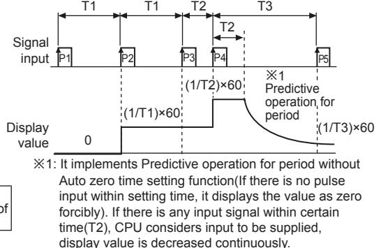
※ 1: It implements Predictive operation for period without Auto zero time setting function (If there is no pulse input within setting time, it displays the value as zero forcibly). If there is any input signal within certain time (T2), CPU considers input to be supplied, display value is decreased continuously.
