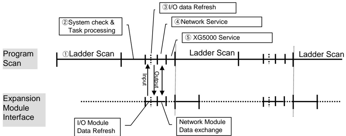
Scan time = ① Scan program process + ② System check & Task process + ③ I/O data Refresh + ④ Network Service + ⑤ XG5000 Service + ⑥ User Task Program process
