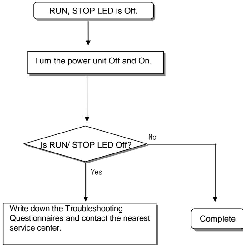
15.2.4 Troubleshooting flowchart used when the I/O part doesn't operate normally.
