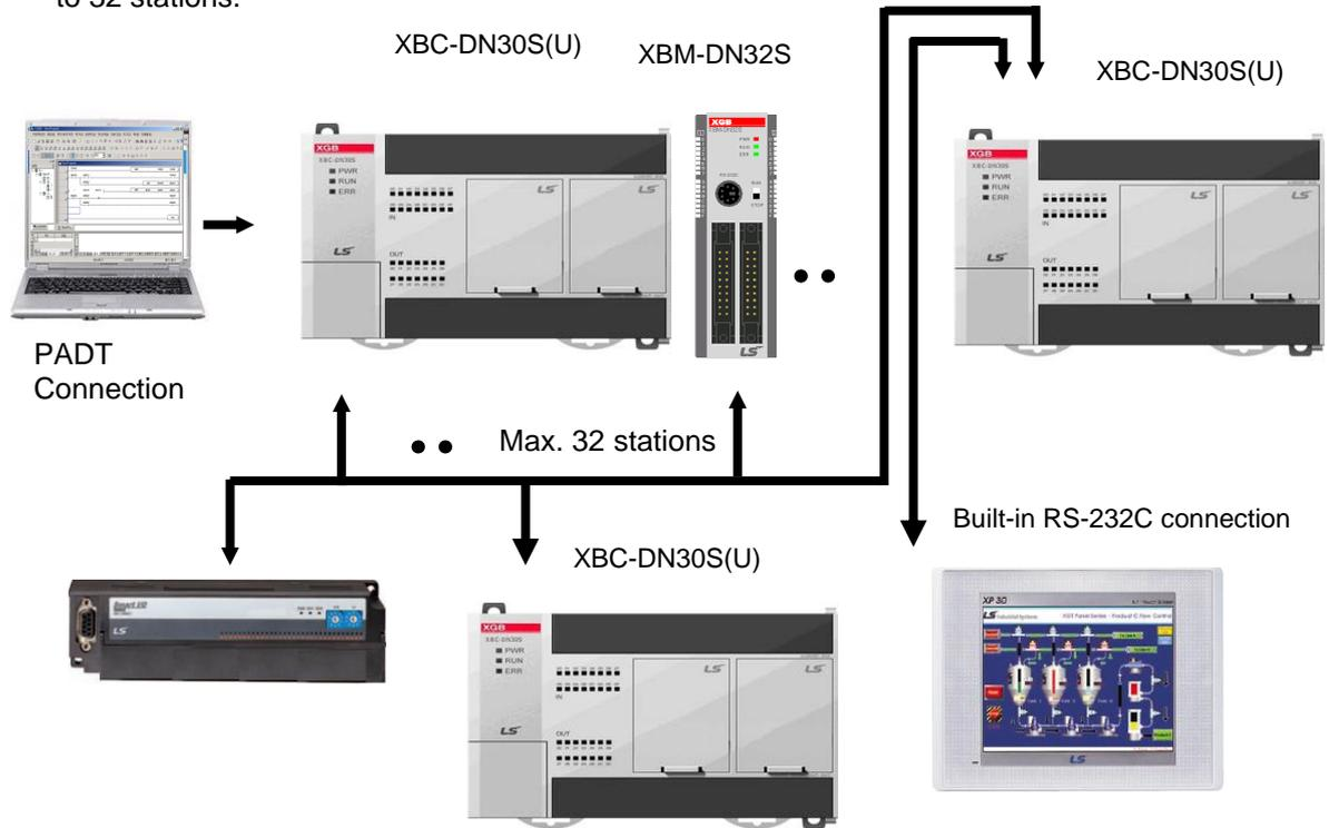
(b) Using RS-485 built-in function/expansion Cnet I/F module can be connect for up to 32 stations.
