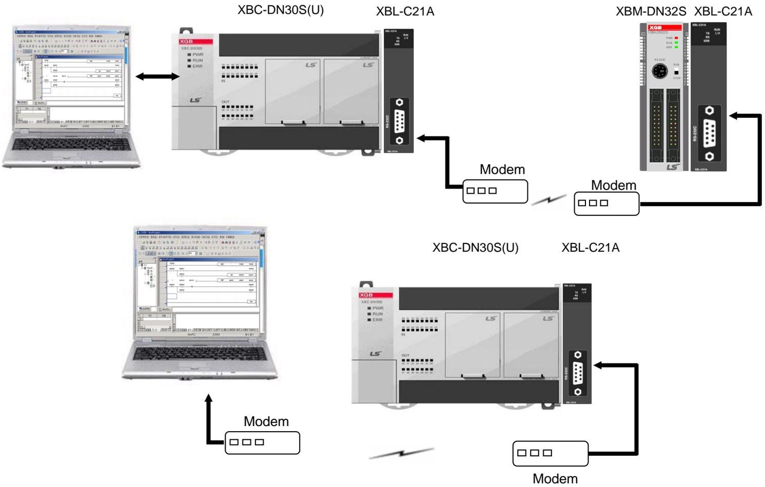
(d) 1:1 communication of an external device (monitoring unit) with main unit using a built-in RS-232C/485 port.
