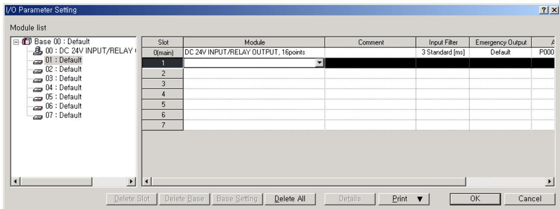
Clicking 『Details』 in 『Slot Position』 shows the following window to set filter and emergency output.
