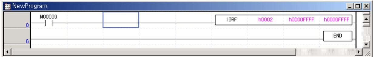
'IORF' command is operated when M00000 is ON. First operand designates slot number. Second operand designates the upper 32 bit data as mask data. Third operand designates the lower 32 bit data as mask data. The bit to refresh set as 1 (hFF) and others set as 0 (h00) (not refreshed).
