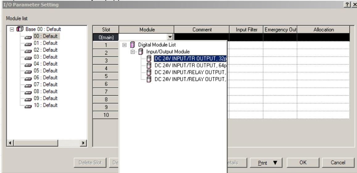
4) After setting I/O module, click Input Filter.
