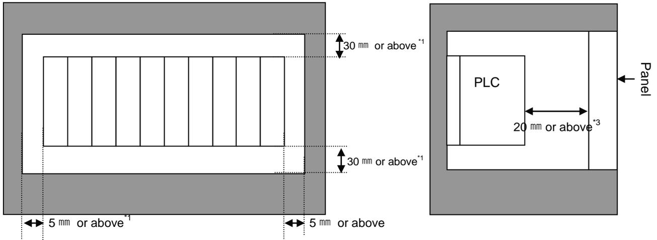
\*1 : In case height of wiring duct is less than 50 mm (except this 40mm or above)
