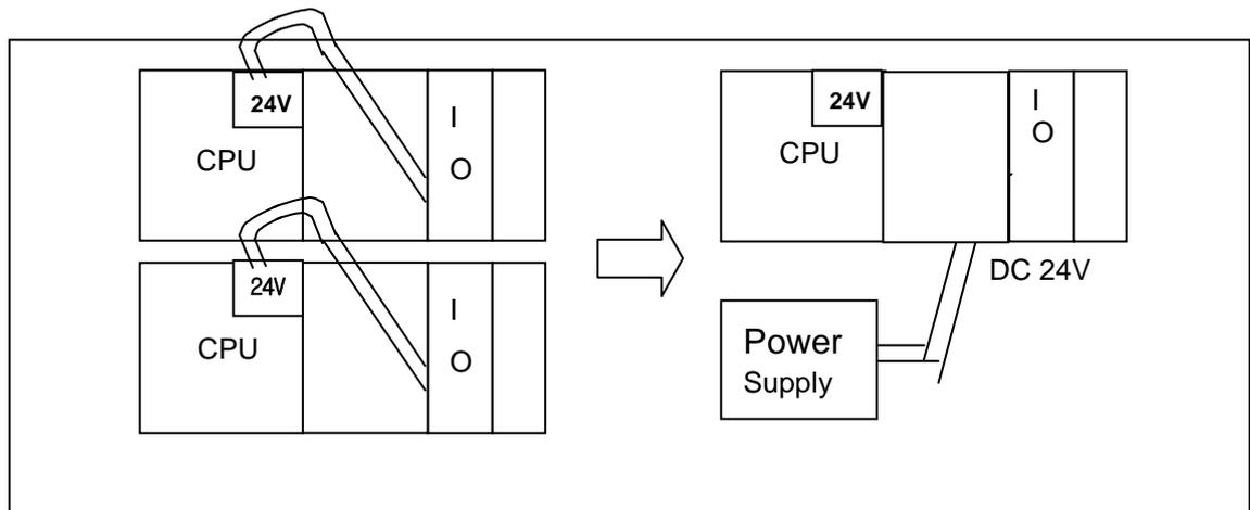
(5) AC110V/AC220V/DC24V cables should be compactly twisted and connected in the shortest distance.
