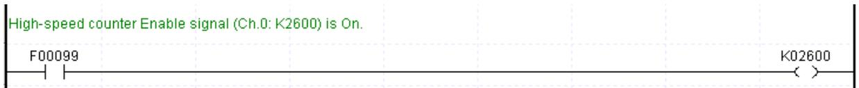
(d) To use additional functions of the high-speed counter, you need to turn on the flag allowing an operation command.
