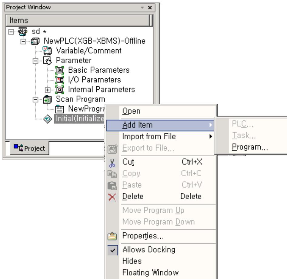
(d) Make initializing program. In initializing program, INIT\_DONE instruction must be made. If not, Scan program is not executed.
