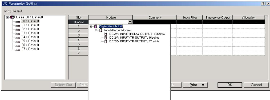
Clicking 『Module』 in 『Slot Position』 indicates a list of modules, in which you may set I/O corresponding to the actual system. Then, the following window is displayed.
