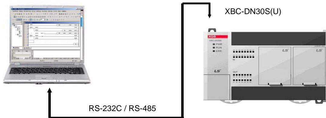
(b) 1:1 communication with main unit using a built-in RS-485 port (In case of built-in RS-232C, it is for connecting to HMI device.)
