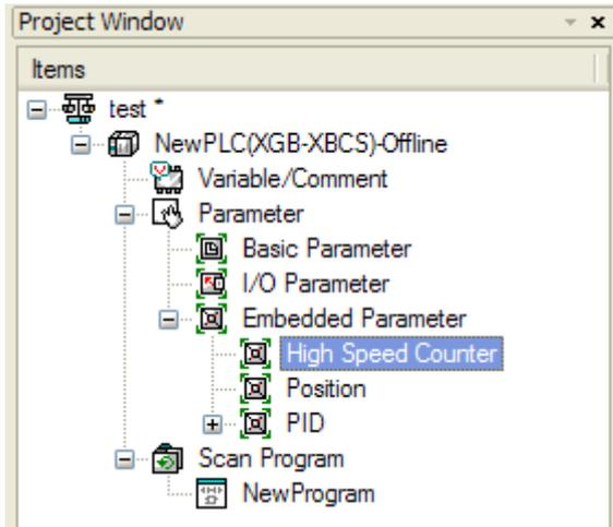
(b) Selecting high-speed counter opens a window to set high-speed counter parameters as follows.
